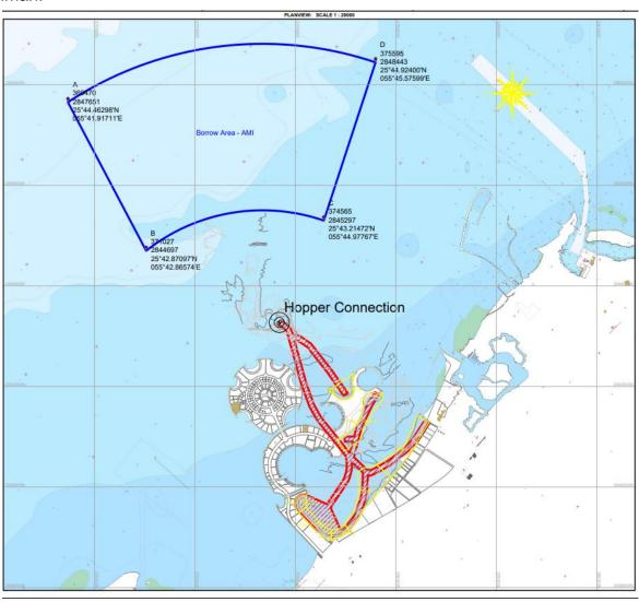
Restricted area of pipeline corridor marked in red. Combination of *Trailing Suction Hopper Dredger Rotterdam* and tugs are all restricted in their manoeuvrability. All vessels will carry their daymarks and navigation lights as such.
