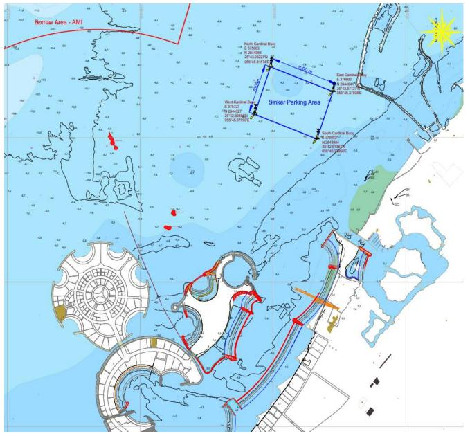
The sinker pipelines will be shifted to the sinker parking area, submerged from 11<sup>th</sup> Apr onwards and remain there for approx. 03 months.
