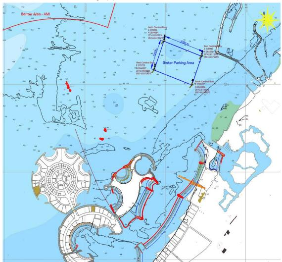
The *Restricted Draft Area* of the pipeline will be designated with Cardinal Buoys as indicated on the drawing, as the water depth decreases due to the pipeline on the seabed. Locations and visual representation of the Cardinal Buoys are detailed in the table below.
